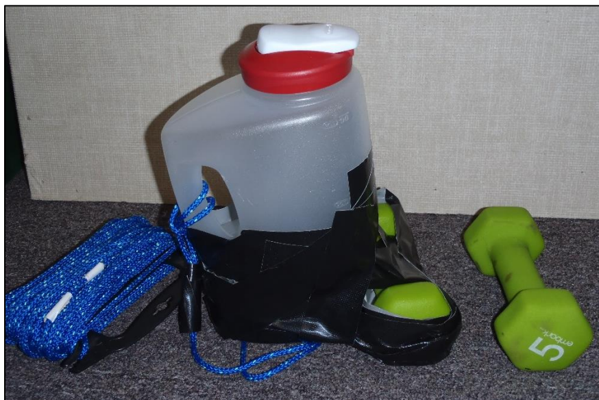
Fig. A3. Sampling container for stream water sampling. The container is 3qt. with a 5lb vinyl coated hand weight taped at the side opposite the handle.
